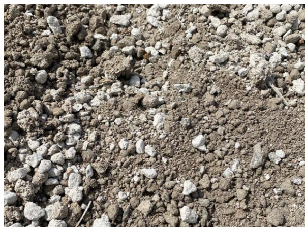
Figure 3.2. Crushed concrete aggregate (0-16 mm)
