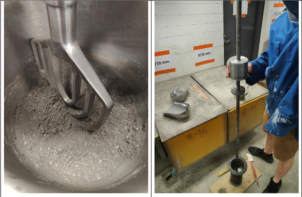
Figure 4.5. Mixing of ingredients in Hobart Mixer (Left); Specimen preparation by using VTT hammer to compact the stabilized rammed earth mixture in mould (Right).
