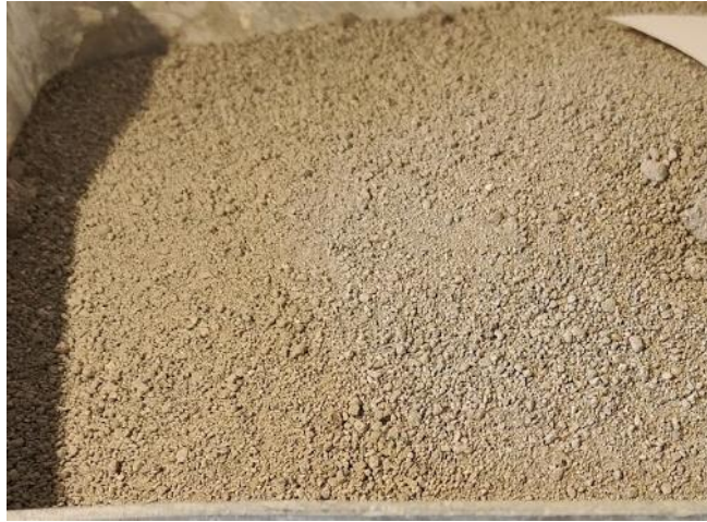
Figure 3.1. Dried incineration slag 0-2 mm
