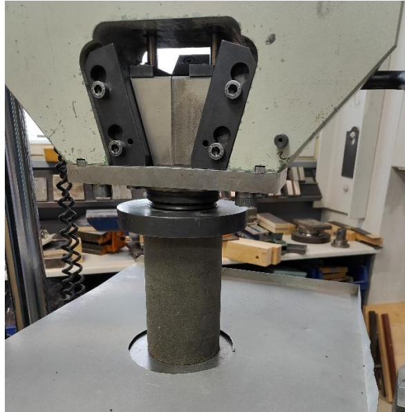
Figure 4.8. Zwick & Roell Uniaxial Compression Test setup, Aalto University
