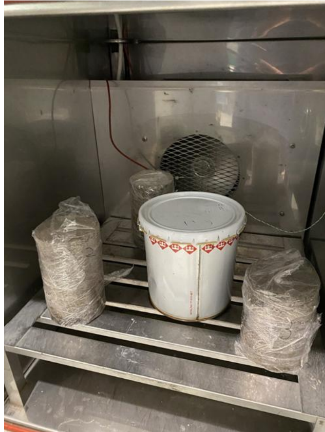
Figure 4.6. Freeze-thaw chamber with test samples.
