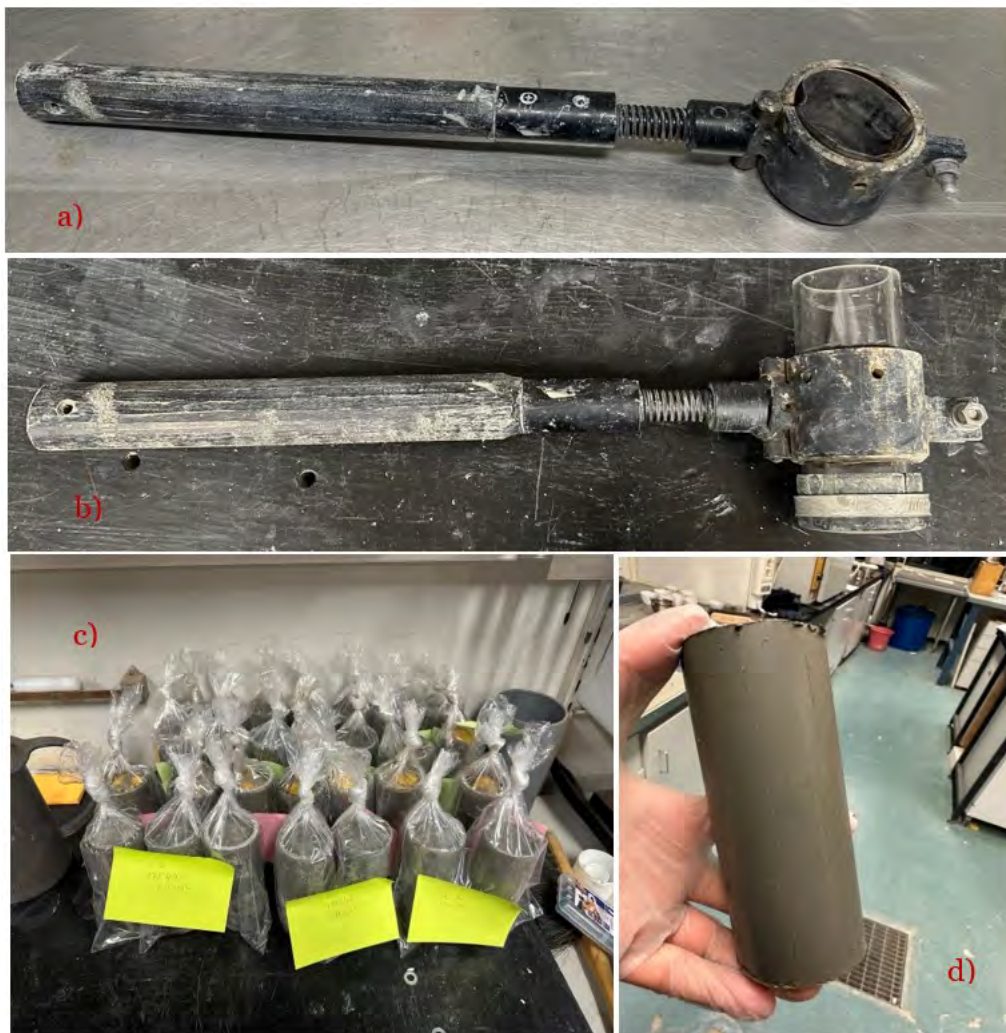
Figure 20. (a) The tool that is used as a hammer, (b) The tube is replaced into the hammer, (c) Samples into the plastic bags (d) The sample after extraction from the tube.
