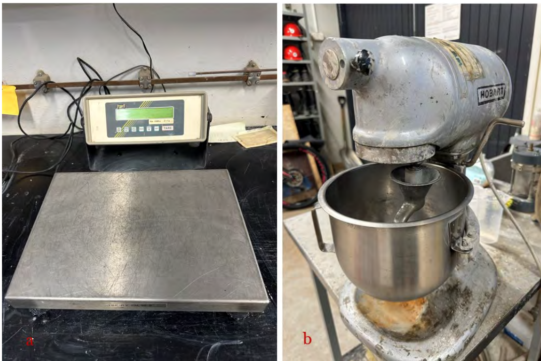
Figure 19. (a) The scale which was used for measuring the weight of the clay and binders, (b) The mixer which was used for mixing the clay and binders.
