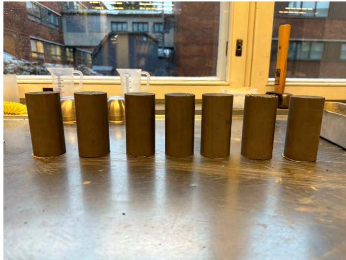
Figure 21. Trimmed samples to 100 mm height.
