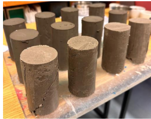
Soil-biochar composites after CO 2 precipitation (use in soft clay stabilization)
