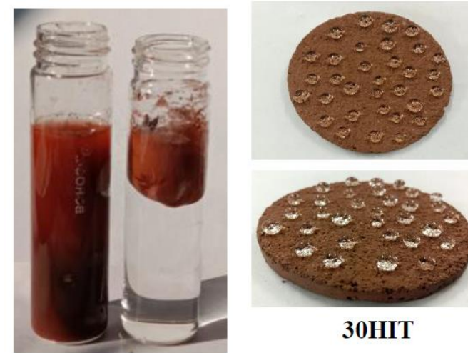
Fig. Hydrophobization of tailings through fatty acids impregnation and use as fillers for hydrophobic mortars
