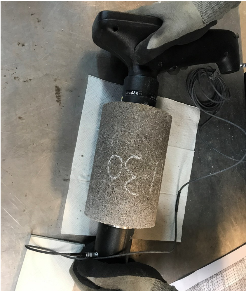
Figure 5.5. Measuring with UPV device.
