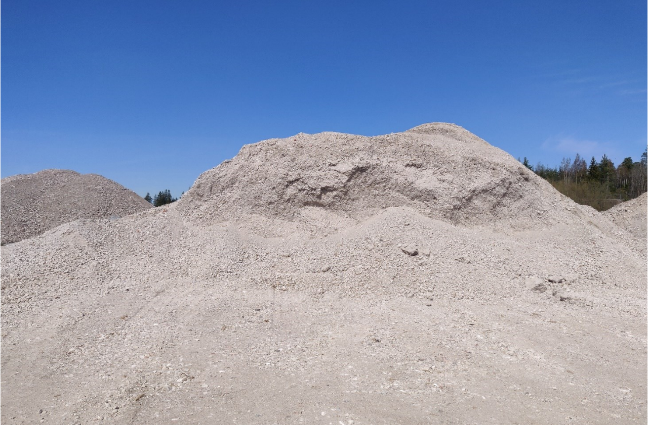
Figure 4.2. Crushed concrete (0-63 mm) at Kiertomaa Oy Saramäki site.
