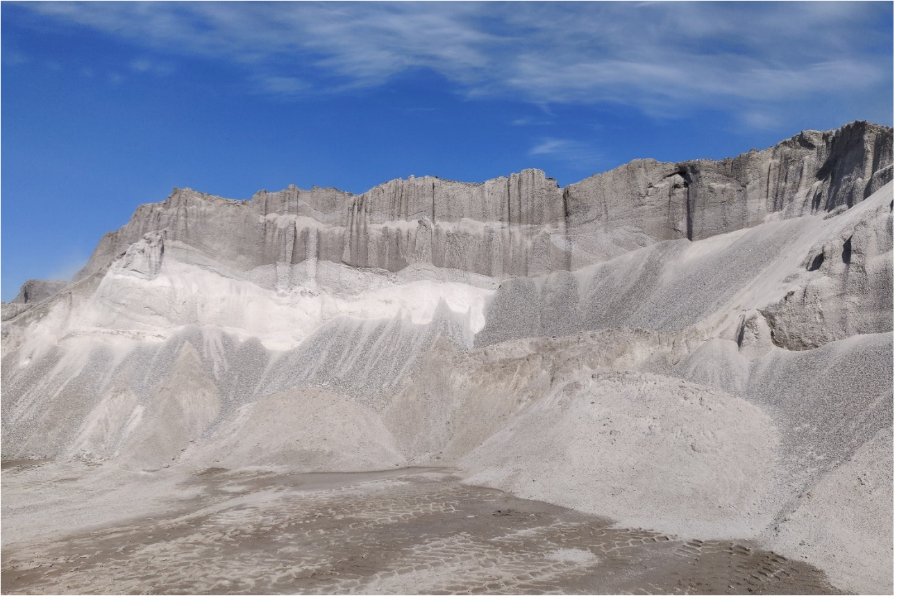
Figure 4.1 Quarry fines (0-5 mm) at Kiertomaa Oy Saramäki site.
