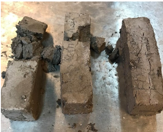
Figure 6.2. Naantali FA samples after demolding.
