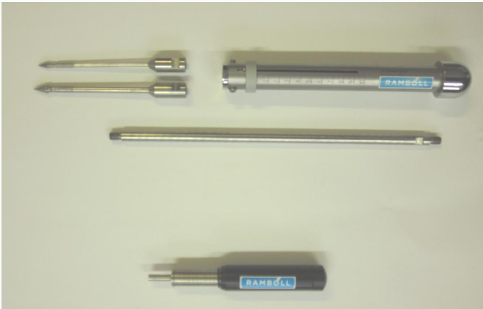
Figure 3.13 Hand penetrometer and pocket penetrometer from Ramboll Oy.
