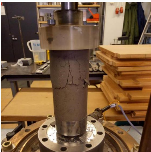
Figure 4.3 Cracks of stabilized clay column in compression test, HELEN + cement (100+50 kg/m 3 ), 3 months (photo Tianlingzi Xiong 11.07.2018)
