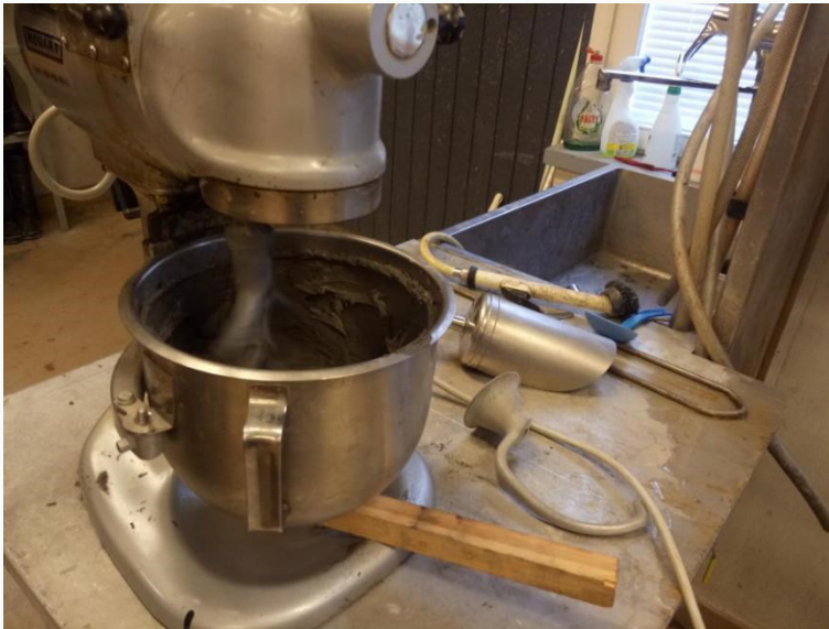
Figure 3.9 Mixing machine used in the mixing of the clay and binder (photo Tianlingzi Xiong 20.03.2018).
