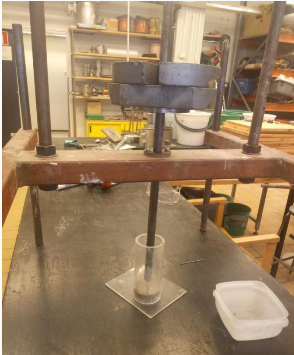
Figure 3.12 Static compaction (photo Tianlingzi Xiong 21.03.2018)
