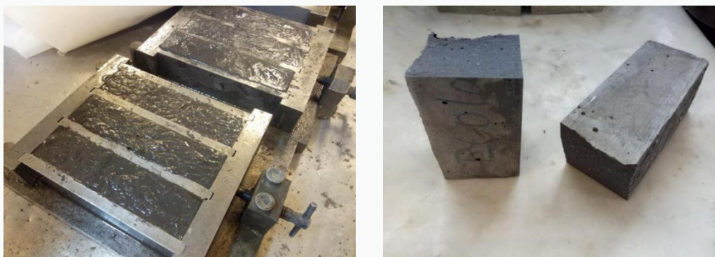
Figure 3.17 Ecolan Ash mixture slurry casting and casted specimens after bending test (photo Tianlingzi Xiong 25.04.2018).
