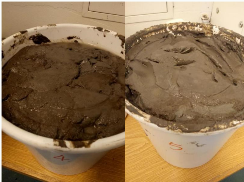
Figure 3.1 Depot of Vuosaari. Soft clay samples in buckets, depth 3.0-3.3 m (photo Tianlingzi Xiong 26.02.2018).
