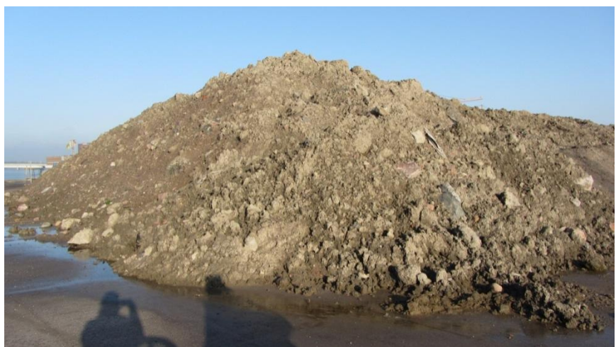
Stabilized and piled sediment
